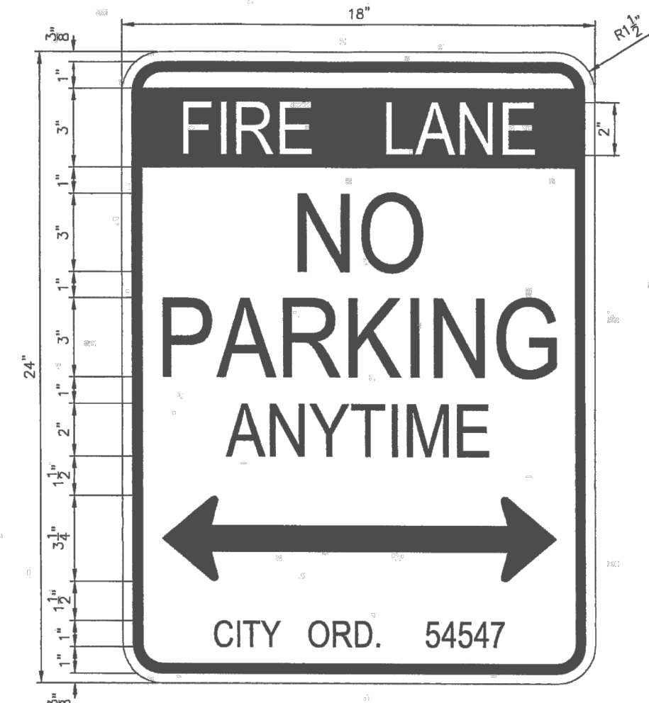
FIRE LANE SIGNAGE
